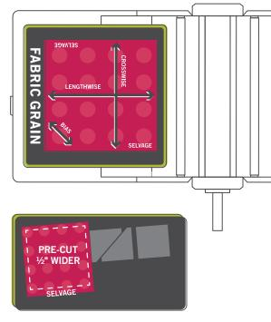
3. SAVE YOUR FABRIC! – When laying your fabric on the die, only place it right over the shapes you wish to cut. There is no need to cover the entire board. Two Tone™ – Foam makes it easy to align fabric just over the edge of the shape so you can save fabric.
